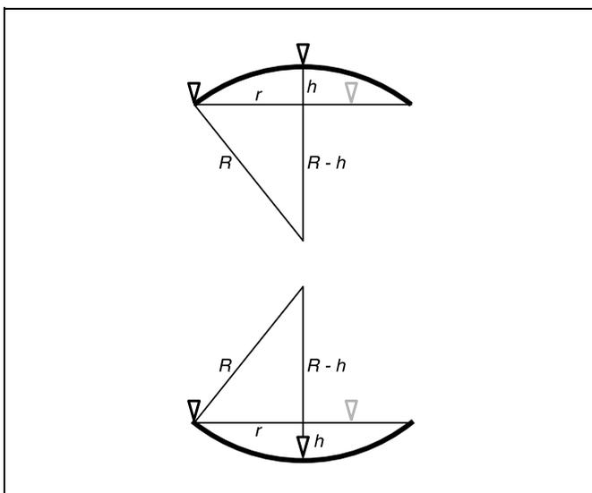
Fig. 1 Measuring the bending radius of a watch glass using a spherometer
